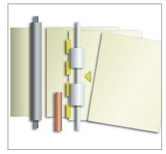
To ensure extremely accurate sheet-to-sheet registration, the RICOH Pro C900/C900s physically adjusts each sheet for skew, position and alignment, and automatically changes rotation speed to compensate for minor differences in timing created by these adjustments.
