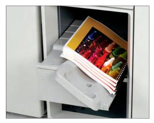
In-line ring binding eliminates the time and expense of inserting binding elements off-line, dramatically reducing labor costs.
