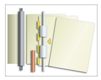
To ensure extremely accurate sheet-to-sheet registration, the LANIER Pro C720/C720s physically adjusts each sheet for skew, position and alignment, and automatically changes rotation speed to compensate for minor differences in timing created by these adjustments.
