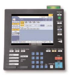
The easy-to-use Operation Panel simplifies access to job functions, including the built-in EFI<sup>™</sup> Fiery<sup>®</sup> print controller.
