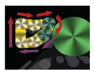
Minimize color density fluctuation across printed sheets and throughout large volume print runs with Single Direction Development. This method prevents reuse of developer after toner is consumed in the development process.
