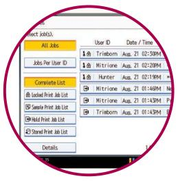
With the available **Locked (Secure) Print** function, users can suspend document printing until a password is entered at the device to release the document.
