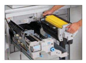
All systems feature Trained Customer Replaceable Units (TCRUs), which trained operators can replace quickly to maximize uptime without calling for service.
