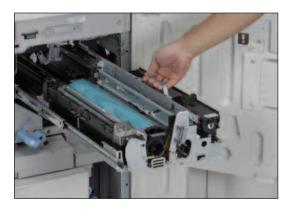
All three systems feature eight Trained Customer Replaceable Units (TCRUs), which trained operators can replace quickly and easily to maintain maximum uptime in certain environments.
