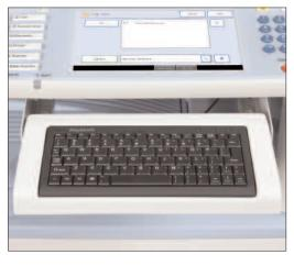
The optional keyboard provides an alternative way to enter data at the device.\*
