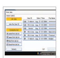
**Locked (Secure) Print** lets users delay document printing until they enter a password at the device.
