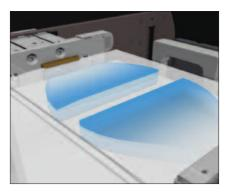
The Air-Assist Media Feed Mechanism blows air between individual sheets to counteract static cling and eliminate multi-feeds, making it easy for you to run more jobs that require coated media.
