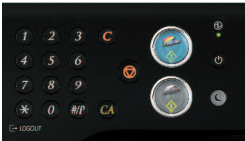
Separate print buttons for B&W and Color allow users to selectively manage use of color
